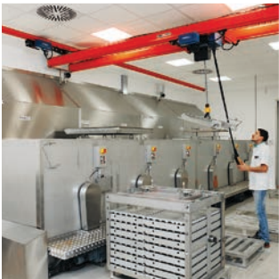
Final pasteurization step of albumin: racks with filled vials are dipped and rotated in a heated water bath
