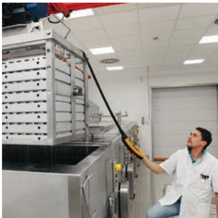
Final pasteurization step of albumin: racks with filled vials are dipped and rotated in a heated water bath
